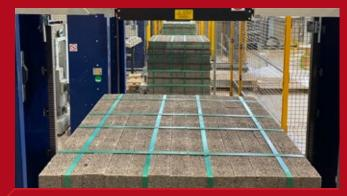
First cubes of UK concrete coursing brick passing through the strapping line.
