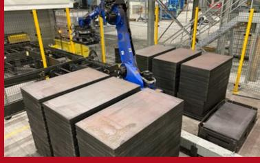
Robotic Buffer Accumulation of up to 510 Pallets.
