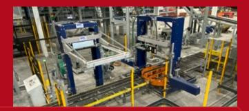
The first of two sets of horizontal and vertical OMS strapping machines.
