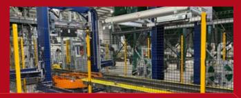
The second of two horizontal and vertical OMS strapping machines in the Columbia automatic cube strapping and stretch plastic film hooding line.
