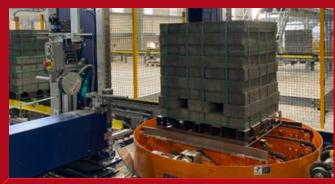
A cube of voided UK concrete coursing brick (with horizontal and two side vertical strapping) leaves the Stowell strapping line on a slave strapping pallet.
