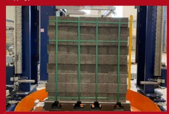
A strapped cube of UK concrete coursing brick ready to receive a plastic stretch film cover.
