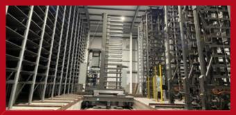
Columbia 18 Tonne PTS with Turntable, Green Side Stacker, 2 x Buffers, 2 x Dry Side Unstackers + CDS Chamber Racking System for 7,000 Pallet Capacity.
