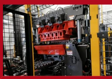
Columbia CPM+60 Concrete Products Machine for Steel Pallet 1400mm x 700mm x 15mm
