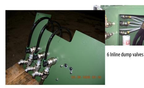
Another way to install 6 dumps. Make sure they are installed as shown as the direction of flow matters.
