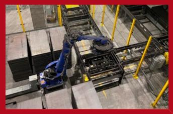
Twin Dry Side Pallet Return, Lift Blade Push-Offs, Brush, Grinding and Pallet Turn-Over To Robotic Buffer Accumulation of 510 Pallets.
