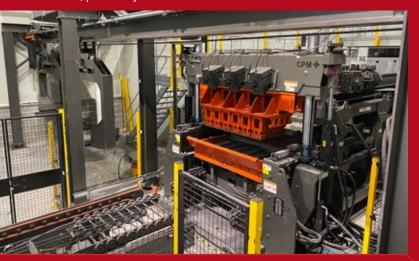
Twin Cassette Fully Automatic Mould Change Inside a Generous CDS Sound Room with 2.5 Tonne Overhead Crane and Targeted Dust Extraction.
