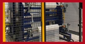
Stretch hooding machinery automatically fits a plastic stretch film cover over final cube.
