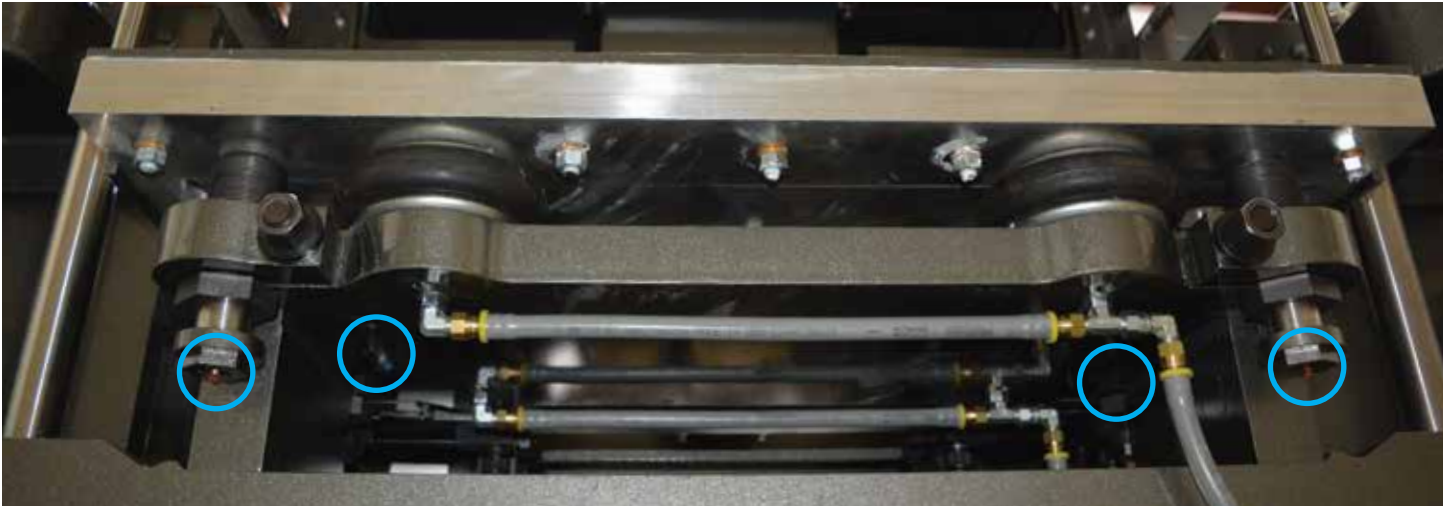
4 grease points (2 front & 2 rear)
