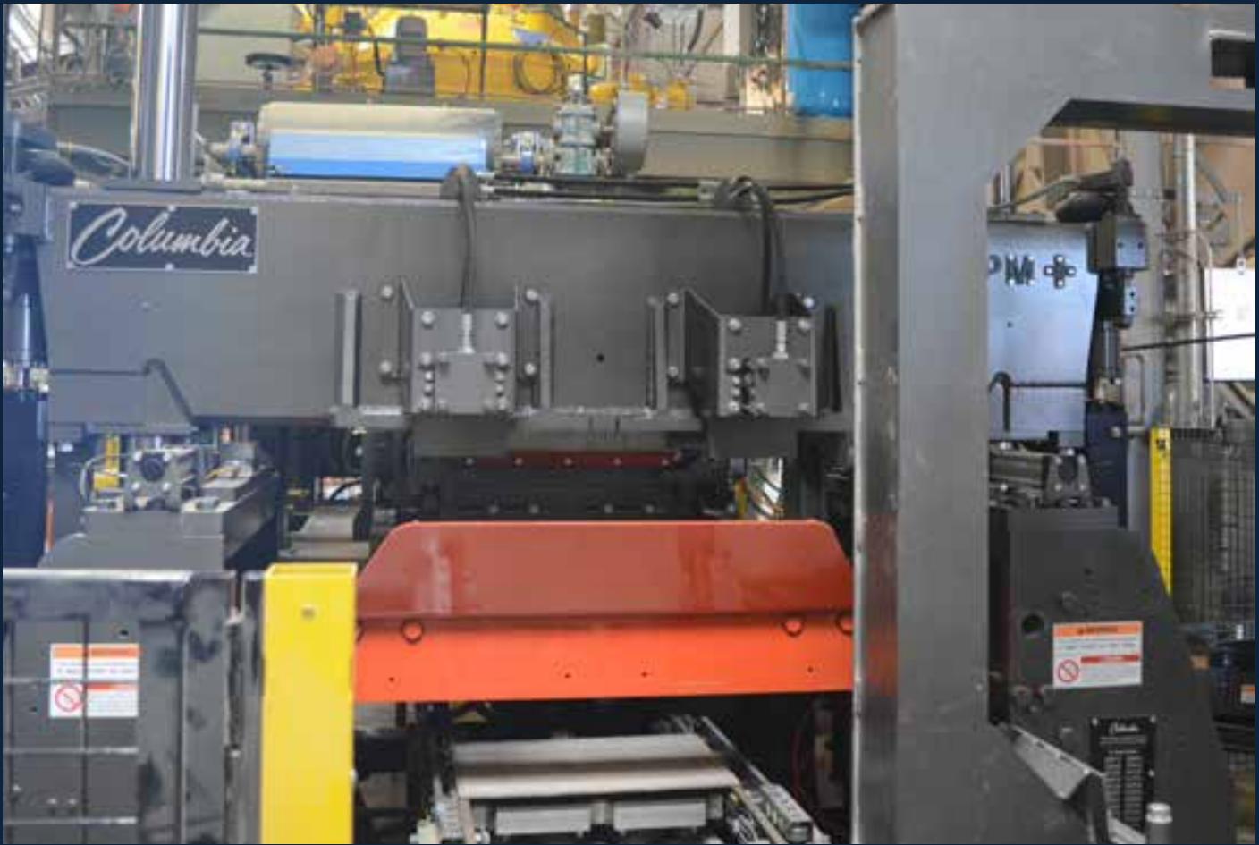
CPM+30 W/ SINGLE CARTRIDGE, FULLY AUTO-MATIC MOLD AND HIGHT CHANGE
