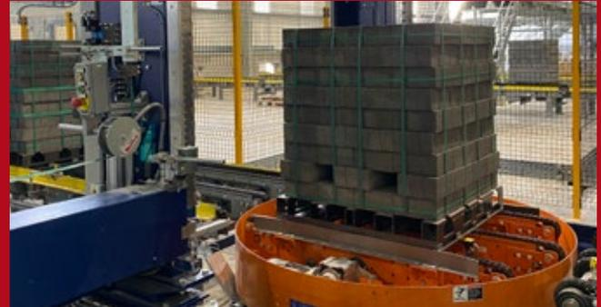
*A cube of voided UK concrete coursing brick (with horizontal and two side vertical strapping) leaves the Stowell strapping line on a slave strapping pallet.*
