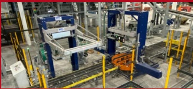
*The first of two sets of horizontal and vertical OMS strapping machines.*
