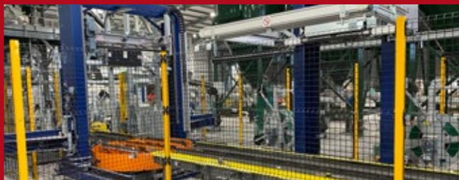
*The second of two horizontal and vertical OMS strapping machines in the Columbia automatic cube strapping and stretch plastic film hooding line.*
