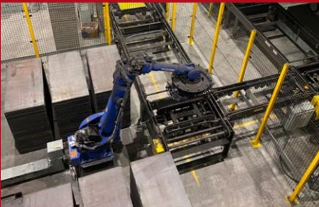
*Twin Dry Side Pallet Return, Lift Blade Push-Offs, Brush, Grinding and Pallet Turn-Over To Robotic Buffer Accumulation of 510 Pallets.*
