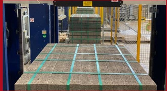
*First cubes of UK concrete coursing brick passing through the strapping line.*
