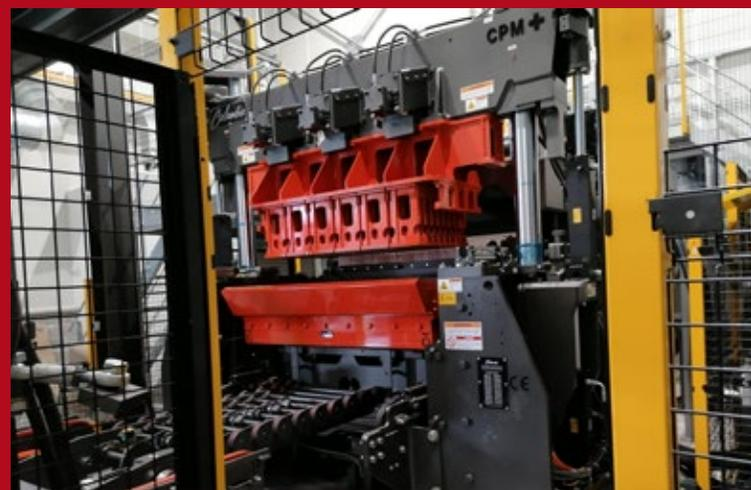
*Columbia CPM+60 Concrete Products Machine for Steel Pallet 1400mm x 700mm x 15mm*
