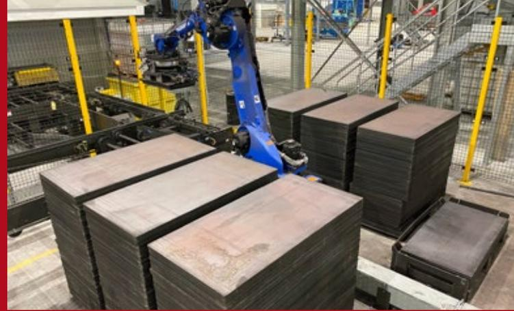
*Robotic Buffer Accumulation of up to 510 Pallets.*
