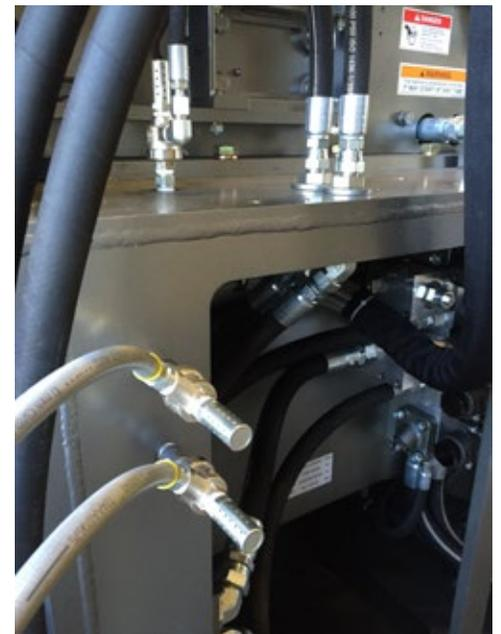
Another way to install 6 dumps. Make sure they are installed as shown as the direction of flow matters.
