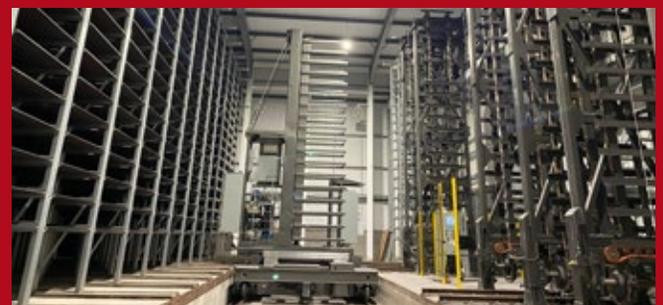
*Columbia 18 Tonne PTS with Turntable, Green Side Stacker, 2 x Buffers, 2 x Dry Side Unstackers + CDS Chamber Racking System for 7,000 Pallet Capacity.*
