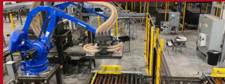
*Vacuum Product Cubing Robot with Columbia Slave Pallet Strapping and Hooding Circuit.*
