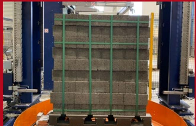
*A strapped cube of UK concrete coursing brick ready to receive a plastic stretch film cover.*
