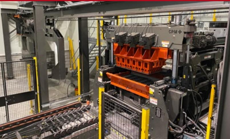
*Twin Cassette Fully Automatic Mould Change Inside a Generous CDS Sound Room with 2.5 Tonne Overhead Crane and Targeted Dust Extraction.*
