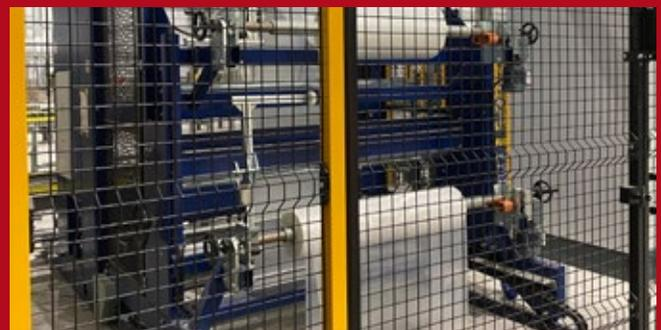
*Stretch hooding machinery automatically fits a plastic stretch film cover over final cube.*
