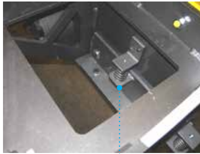
Rear seal spring mount.
