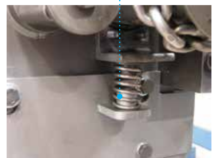
Front spring side seal.
