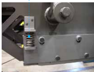
Rear spring side seal.
