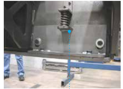
Rear seal spring mount.
