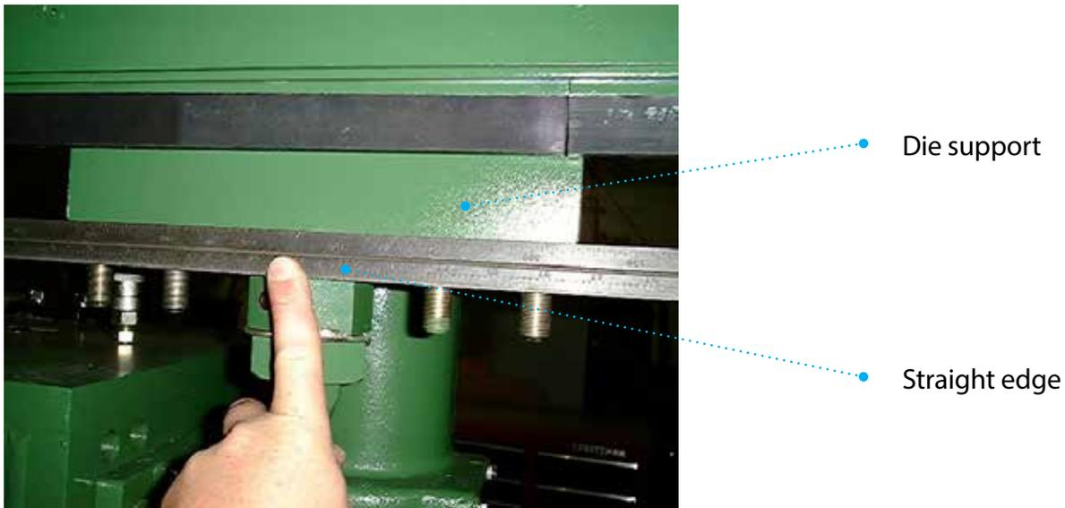
**After inspecting the mold, replacing parts and realigning, install the mold.**
