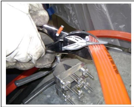
2. Notice the nylon cord in the pictures below. After cutting the belt make sure you have some gloves on when drilling out the nylon cord on both ends of the belt. (See photo below). Again using the VAR welding instructions and for non-reinforced VAR Belting skip to step 10 on the instruction sheet. If you have the cord, follow steps 3 through 9 of the instructions.
