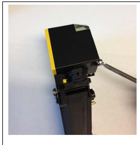
Tighten/Torque screws to 2.0 NM or 1.475 ft. lbs.
