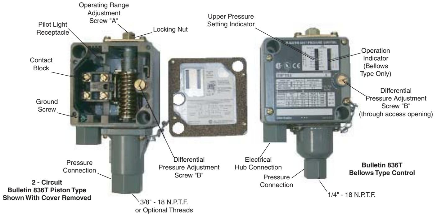
**DESCRIPTION** - Bulletin 836T, Type 1, 4, & 13 oiltight pressure controls are designed for use on machine tool applications where a stream of oil or water may flow over the enclosure. Other applications would include areas where it is desirable to resist the entrance of lint, dust, and dirt into the enclosure.
