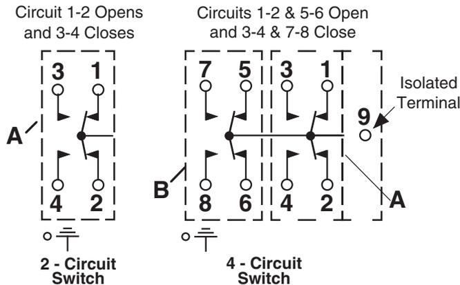
A or B circuits must be the same polarity.
