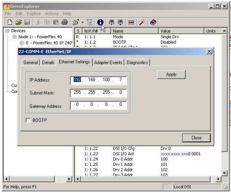
4. Enter the correct EtherNet/IP address and subnet, then click Apply.
