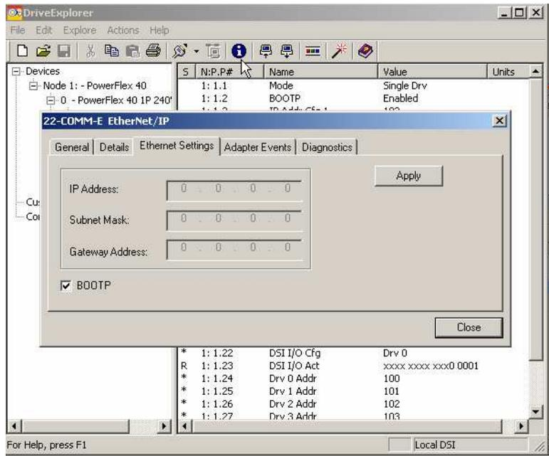
3. Uncheck the BOOTP box, so that the EtherNet Settings are not greyed out and can be adjusted
