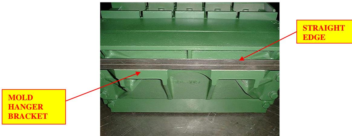
3. To make sure the mold hanger brackets are installed correctly, measure all four corners using a dial caliper, as shown, using the outer holes. Verify measurement of all four corners are the same.
