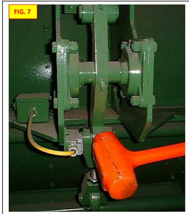
Finally, check the door to see if it is completely closed by using a piece of paper. Try to slide it in between the stop bar on the door and the stop block on the mixer frame. If there is a gap the door is not adjusted correctly. Re-adjust as necessary. (See fig. 8)
