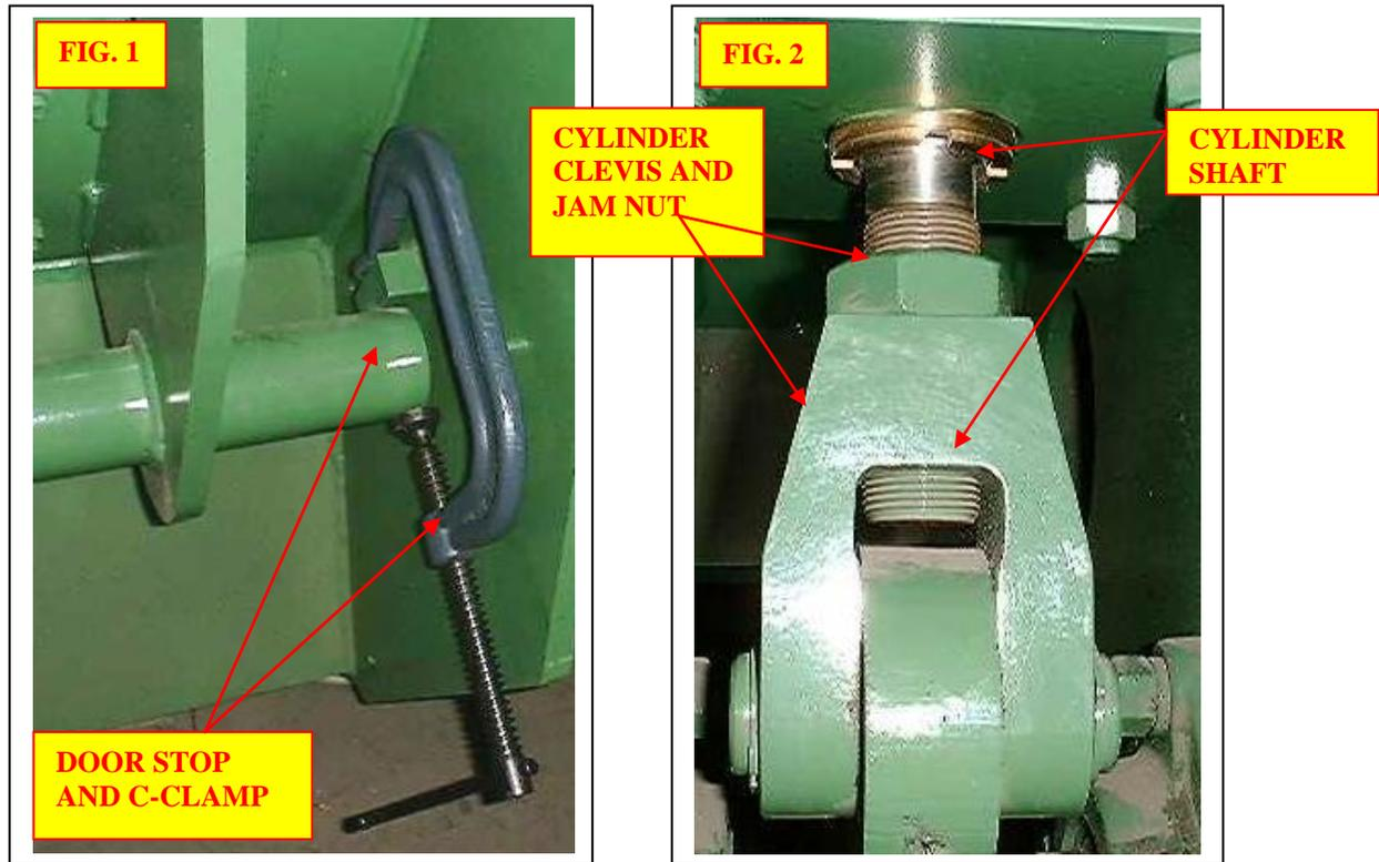
Inspect cylinder for air by-pass: 1) Hook cylinder to air using the base port, leave rod end port open. 2) Extend cylinder, once cylinder shaft has bottomed out listen for leakage. This will check one piston seals for wear. Moving the hose to the rod end port and retract the cylinder, again listen for leakage, this will check the piston and rod seals.
