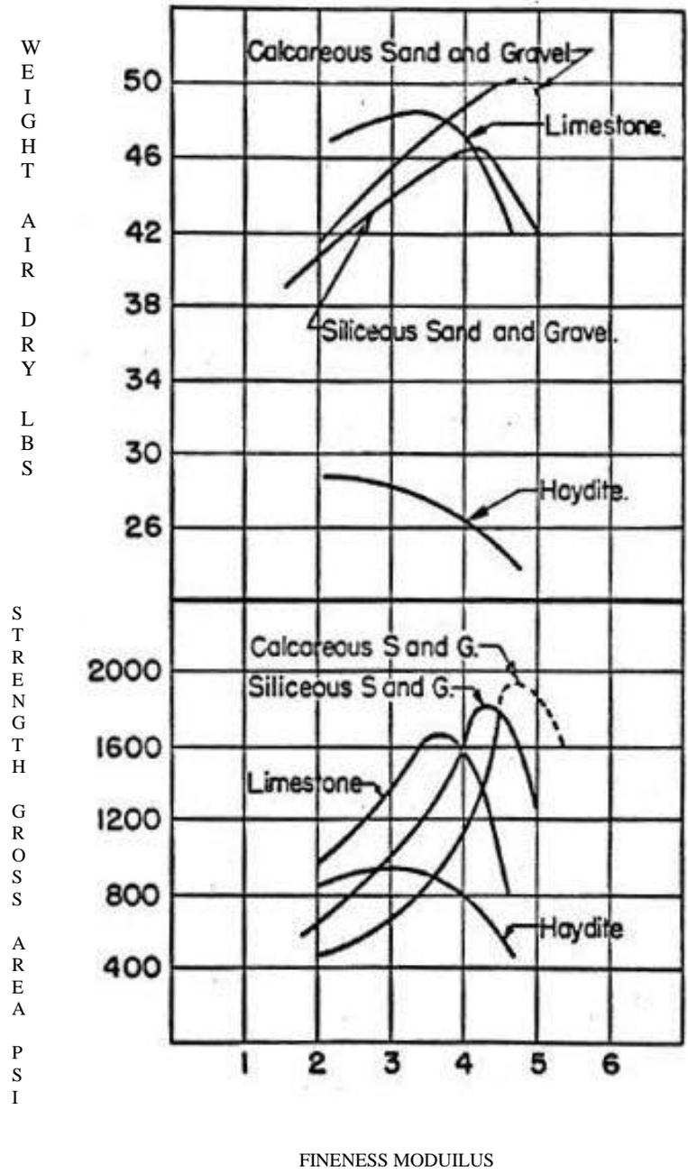
Fig. 2 – Relation of F.M. to Block Weight and Compressive Strength.
