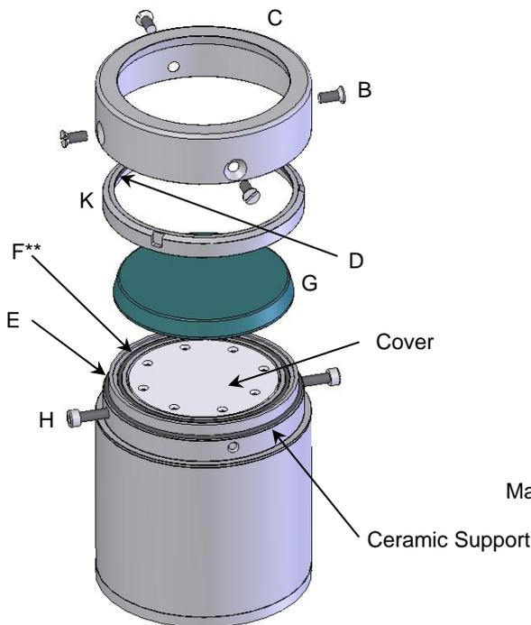
1. Unscrew 4 screws (B) and remove the Protection Ring (C).
