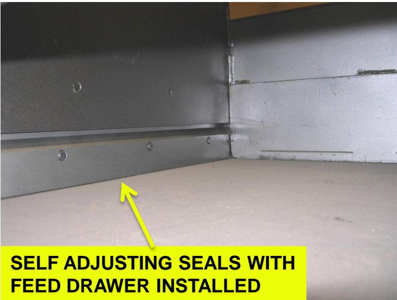
BOTH SIDE AND REAR SEALS INSTALLED
