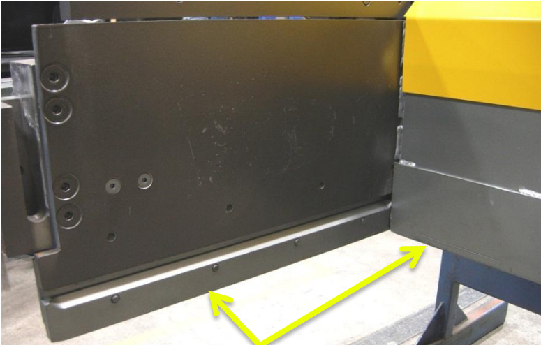
BOTH SIDE AND REAR SEALS INSTALLED
