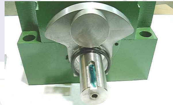
STEP 4 Use 603 loctite in key-way
