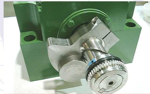
STEP 10 After sliding seal into place on the hub install second set screw with 242 loctite
