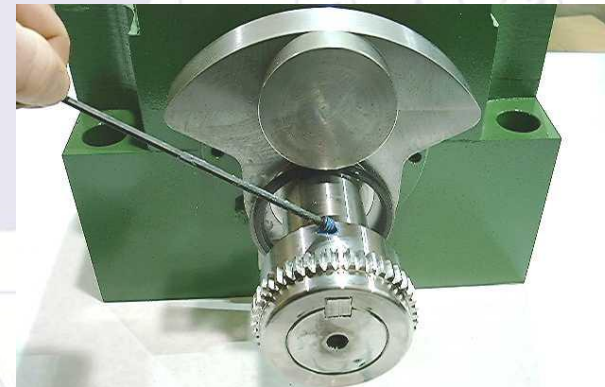
STEP 8 Apply 242 Blue loctite to set screw and hole in key-way, and install this set screw first
