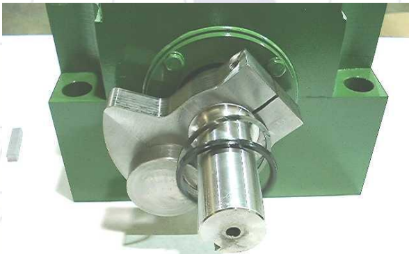
STEP 3 Install snap ring and seal
