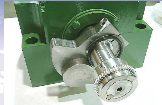
STEP 9 Install first set in other hole using 242 blue loctite
