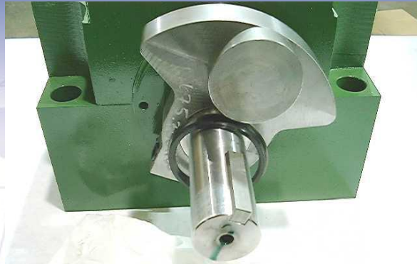
STEP 5 Install key into key-way
