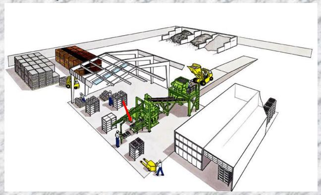
The Block is transported via the Offbearer from the Rollway to a Rack
