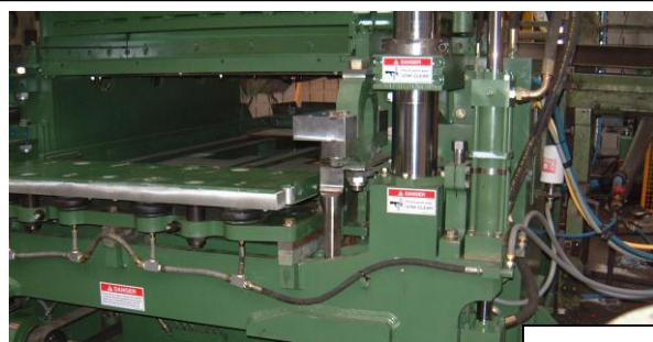
You will notice around each of the bolts on the retainer bracket for the column and the bolts that hold that hold the vibrator to the base of the machine have a bead of blue RTV silicone around them to help eliminate concrete dust or other foreign material from entering these areas. See additional pictures for other areas to seal.
