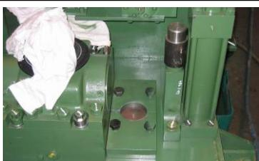
With columns removed it is advised that you clean the base of the machine of all material build up and inspect the column retainers for wear and that all bolts are in good shape. Check to make sure they fit properly with bolts installed.
