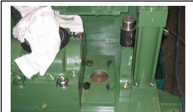
With columns removed it is advised that you clean the base of the machine of all material build up and inspect the column retainers for wear and that all bolts are in good shape. Check to make sure they fit properly with bolts installed.
