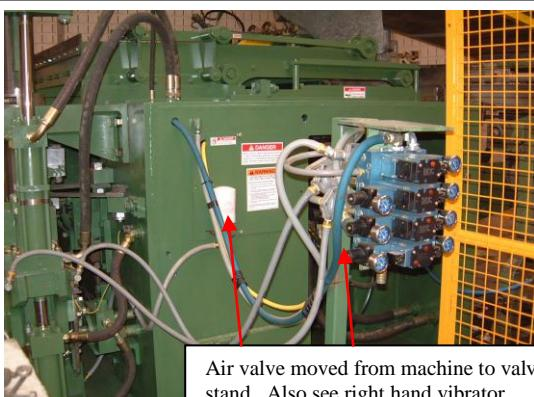
Air valve moved from machine to valve stand. Also see right hand vibrator venting added.
