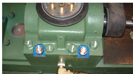
Notice RTV silicone on each lock washer gap. Additionally the white hash marks note these bolts have been torque to proper specks.
