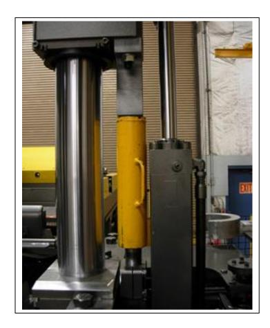
Now turn off pump. With these Safety stops installed, you can now perform maintenance in a safe manner without the beams falling from a mechanical failure or defect. Cylinders can also be removed without stored energy
